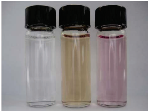
Figure 2. Photograph demonstrating color shifts in water: left: NaPSS brush ( c(\text{NaPSS}) = 240 \mu\text{M} ); center: NaPSS brush with TAPP ( c(\text{NaPSS}) = 240 \mu\text{M} , c(\text{TAPP}) = 30 \mu\text{M} , l = 0.5 ); right: TAPP ( c(\text{TAPP}) = 30 \mu\text{M} ).
